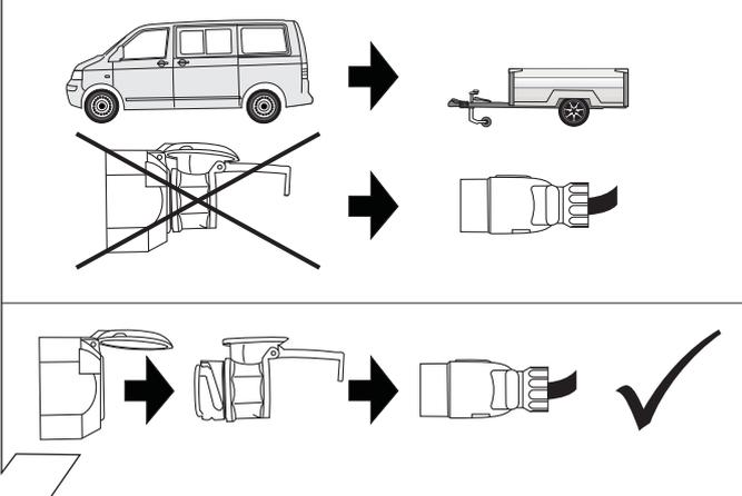
The diagram shows two rows of connections. The top row shows a van connected to a trailer with a 7-pin socket, which is crossed out with a large 'X'. The bottom row shows a 13-pin socket on the van connected to a 13-pin socket on the trailer, which is marked with a checkmark.
