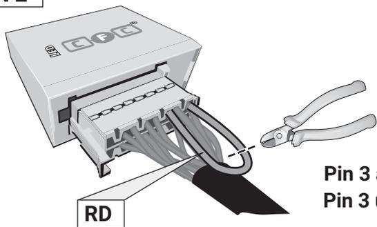
Pin 3 and Pin 2 disconnected
